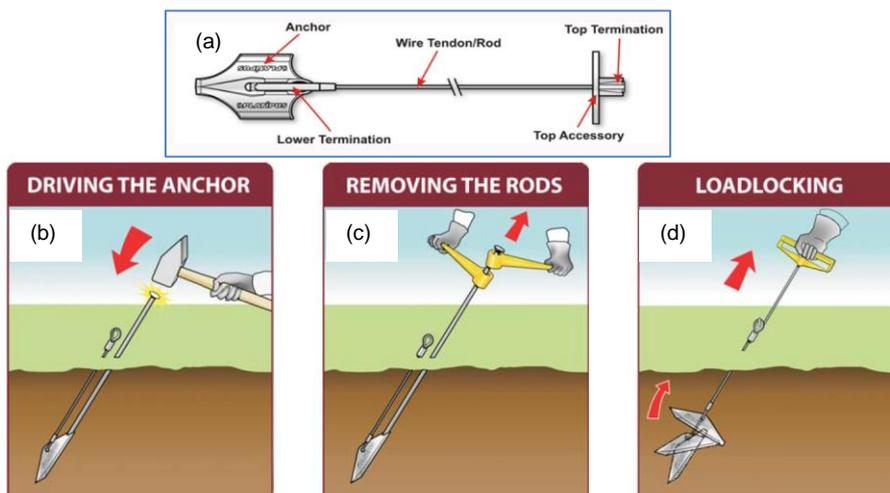
Figure 2: Schematic diagram of Platipus anchors (Platipus Anchor Limited (n.d.))
