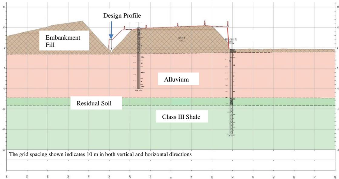
Figure 1: Geological Cross Section of M4 Embankment that required widening
