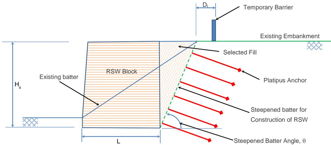
Figure 4: Layout of Temporary Excavations and Anchor Arrangements
