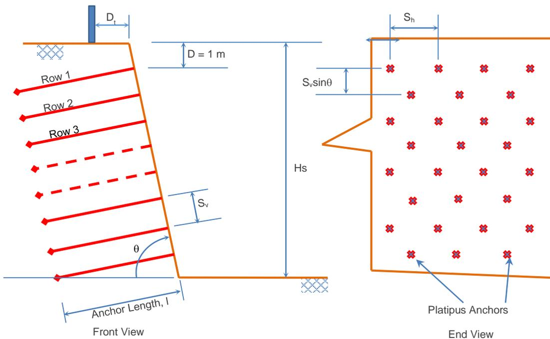
Figure 5: Typical Platipus Anchor Layout in a Temporary Slope
