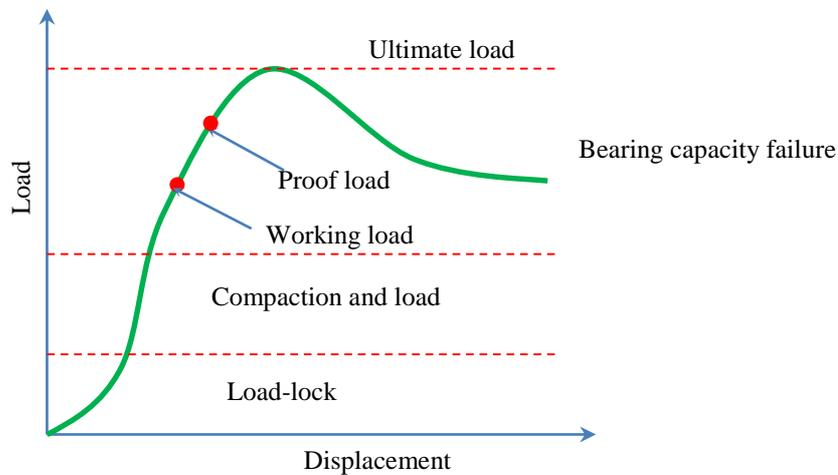
Figure 3: Schematic load-displacement behaviour of Platipus anchor (Platipus Anchor Limited (n.d.))
