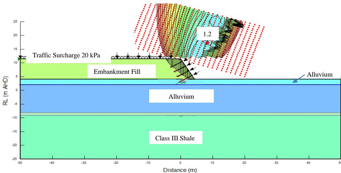
Figure 6: Example Slope stability assessment
